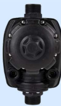
An electronic pressure flow switch automatically controls the start and stop of single-phase electric pumps (surface, vertical and submerged) up to 2 HP. The device starts the electric pump following a decrease in pressure (opening valves) and stops it when the flow of liquid is interrupted at the electric pump's maximum pressure (closing valves).
